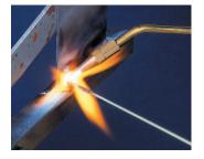
into the joint by capillary action.
